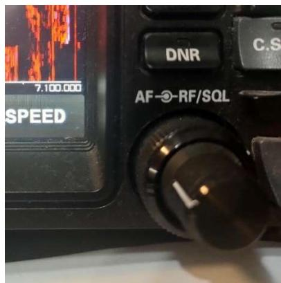
In this mode, instead of **RF**, it is **SQL**. In the other modes - **SSB/CW**, and in **AM**, you will have to rely on your ears and filters. When you are in a mode in which you cannot use a squelch, the knob is an intermediate frequency gain control.
