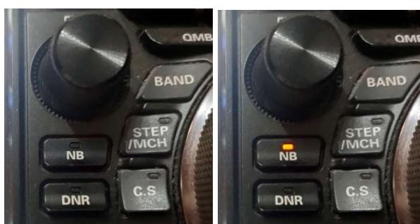
Designed to eliminate "crackling" from ignition of cars, electric fences, switching power supplies, inverters and other converters.
