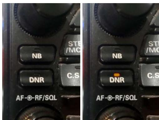
The **DNR system** in the **FTDX10** is legendary. It is extremely effective against atmospheric noise, especially in low ranges (**160m/80m/40m**). It has **15 different algorithms**, the effectiveness of which (strength) does not depend on the size of the number.
